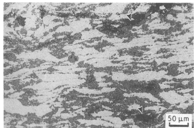
Figure 13 Microstructure of the MMC (as-extruded) deformed at 550 °C and 1 s -1 showing large cracks (arrows).
